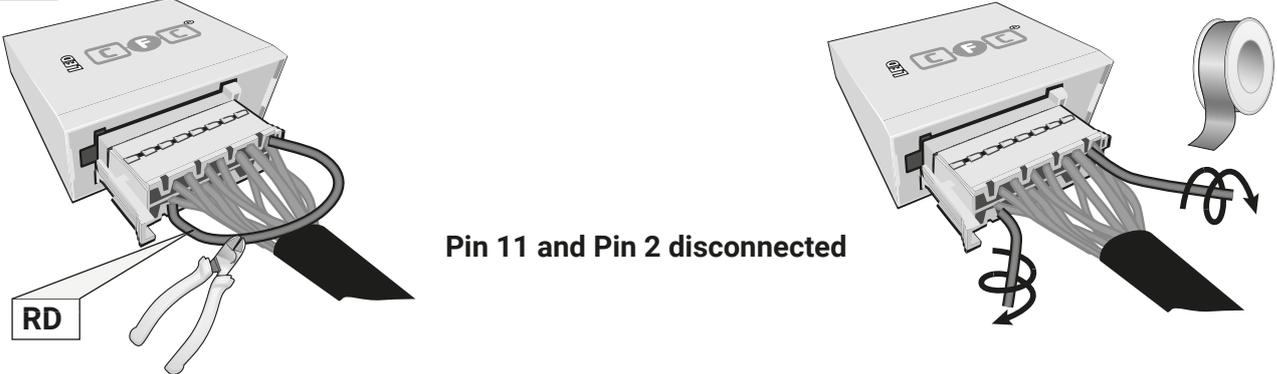
Pin 11 and Pin 2 disconnected
