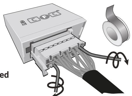
Pin 11 and Pin 2 disconnected
