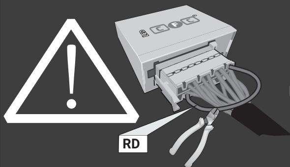
Pin 11 and Pin 2 disconnected
