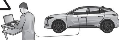
The light functions on the trailer will only operate **AFTER** the vehicle has been re-coded!
