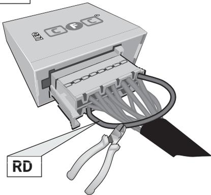
Pin 11 and Pin 2 disconnected
