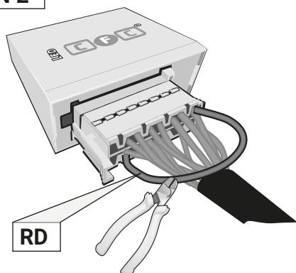
Pin 11 and Pin 2 disconnected
